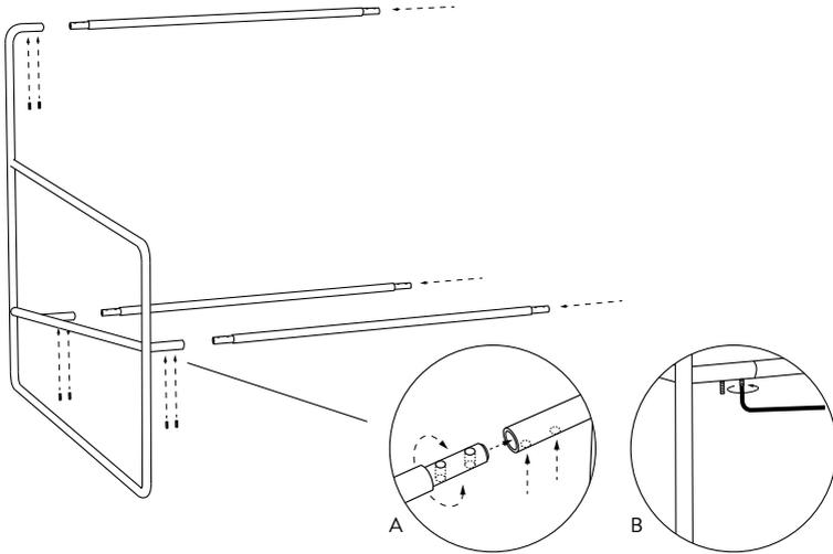
1. Connect the three rods to the left-sided frame (A). Twist the rods to make sure that the screw holes on the rods and on the side frame are aligned (B). Use the included Allen Key to place the screws in the center of each screw hole, and carefully secure each screw **halfway** into the frame. This is important for the following steps.
