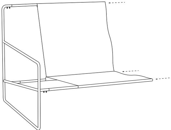
2. Carefully mount the fabric cover over the three rods, making sure that the screws – which are only screwed halfway into the frame – do not rip or damage the fabric.
